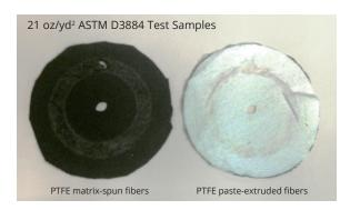
Toray matrix-spun PTFE felt (Brown) can withstand on average 26% longer cycles before breakthrough in abrasion testing compared to PTFE paste-extruded PTFE felt (White). After the abrasion test, the white sample demonstrated wear. The brown felt remained almost completely opaque, showing no sign of wear. (In ASTM D3884; Subject to a Taber abrader with a H22 abrading wheel at 1 kg pressure.)
