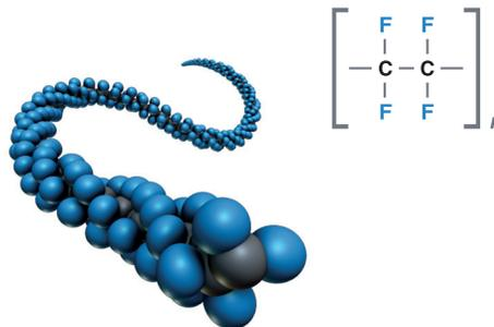
PTFE in its purest form: long chains of carbon atoms (black) tightly saturated with fluorine atoms (blue).
