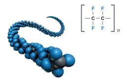
PTFE in its purest form: long chains of carbon atoms (black) tightly saturated with fluorine atoms (blue).
