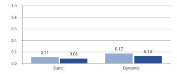
Velocity; Static / Dynamic; 0.00042 / 0.050 m/sec (0.082 / 9.8 ft/min) Based on ASTM D3108
