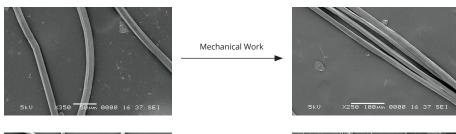
Upon subjecting PTFE matrix-spun fibers to scraping with a knife edge, **no abrasion was observed.**
