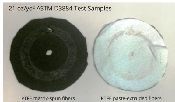
Toray matrix-spun PTFE felt (Brown) can withstand on average 26% longer cycles before breakthrough in abrasion testing compared to PTFE paste-extruded PTFE felt (White). After the abrasion test, the white sample demonstrated wear. The brown felt remained almost completely opaque, showing no sign of wear. (In ASTM D3884; Subject to a Taber abrader with a H22 abrading wheel at 1 kg pressure.)
