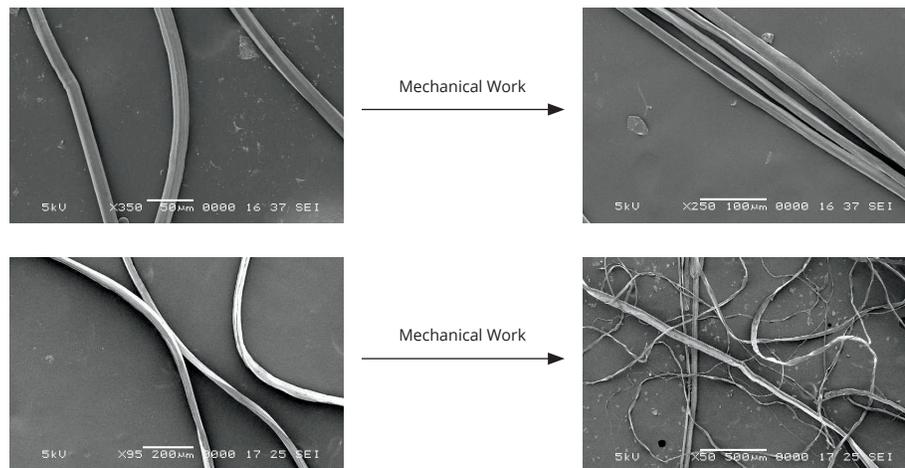
Upon subjecting PTFE matrix-spun fibers to scraping with a knife edge, **no abrasion was observed.**
