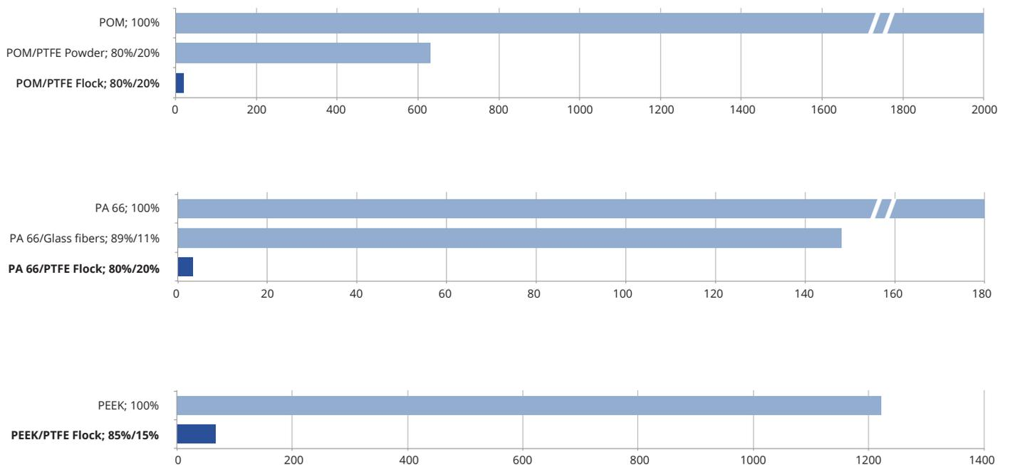
Wear Factor; Shows the Ratio of Wear Volume (Lower Number = Higher Resistance for Wear)
